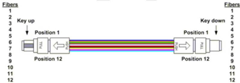
Figure 7 - Type-A:1-1 array patch cord and array cable (key-up to key-down)
