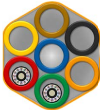
Microducts: 7 x 12.7/10 mm Bundle OD: 1.64 in Micro cable OD: 8.1 mm
