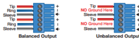
Figure 7. 6-pole Audio Output Wiring
