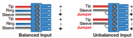
Figure 5. 6-pole Audio Input Wiring
