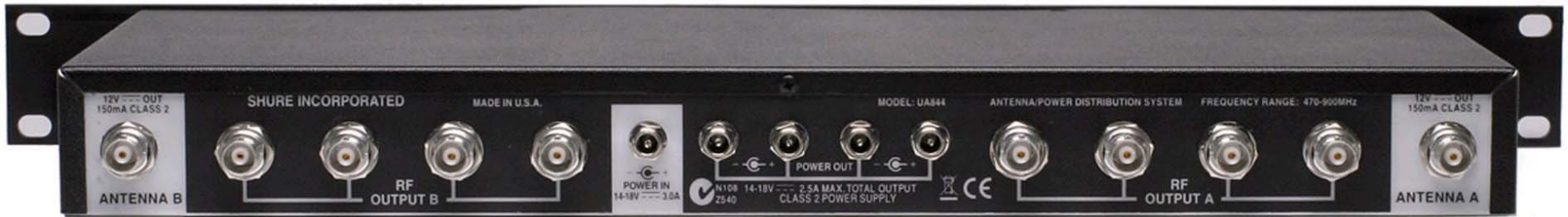
Antenna Distribution Amplifier
