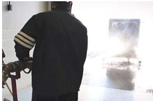
3. Assembly is subjected to hose stream test.
