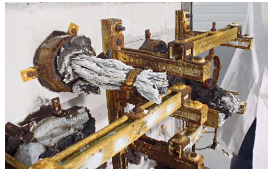
4. Assembly results after hose stream.
