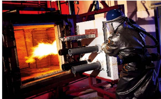
1. Assembly is placed on furnace.
