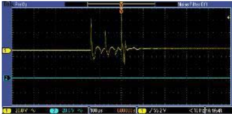
Before & after 60 Hz transient with 6 pair INT in HumZapper
