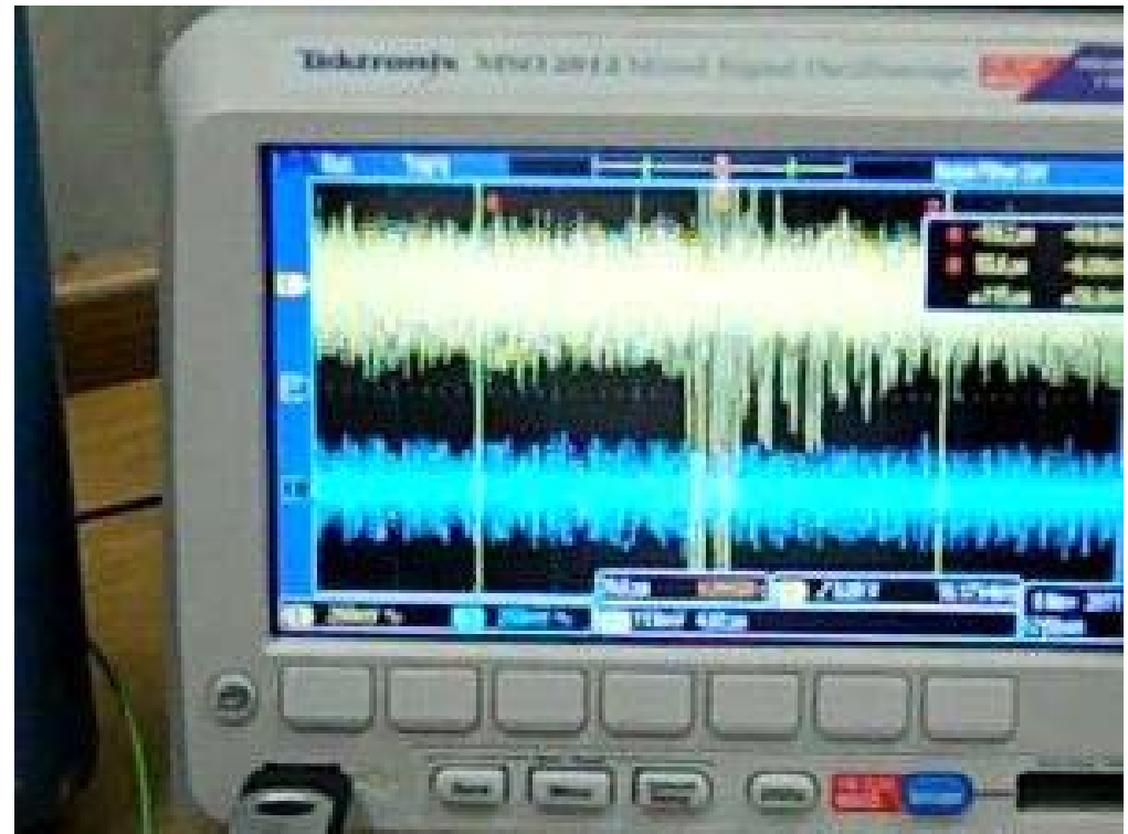
Before & after lightning transients through DSL INT prototype on AT&T Lab U-verse circuit November 8, 2011
